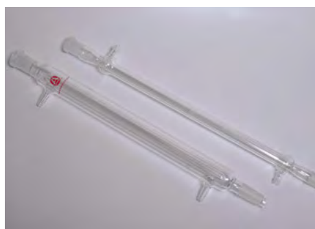
Two Liebig condensers which are used in the distillation process
